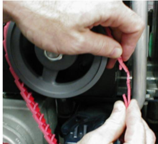
**Figure 4-9 Sizing the Link Belt**
