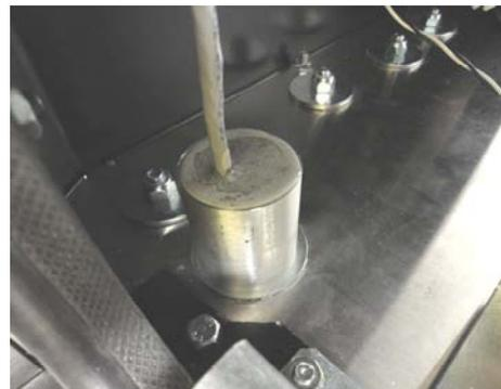
Note: Prepare the potting compound by pouring 4 oz. Rockite into an eight oz. paper cup. Add 1-1/2 oz. of water. Stir one to two minutes until reaching consistency similar to pancake batter. Pour mix into fitting and fill to within 1/8" of top of fitting. Cable should exit near the center of the fitting.
