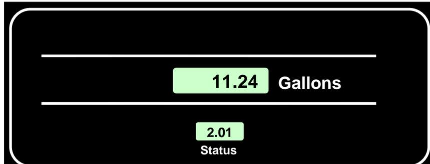
Figure 4-2 In this example, the Status display shows subfunction 2.01 (date) with its value of 11.24 (November 24) shown in the Gallons display.
