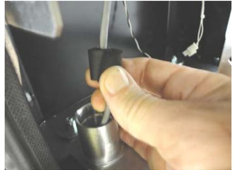
**C** - Wrap Sealing Gasket with tape to hold it in place.
